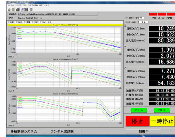
Fig.4 Actual 3-Axis Simultaneous Vibration Random Profile According To MIL-STD-810G Method 514.6 ANNEX C Category 4 –Common carrier (US High way vibration exposure)
