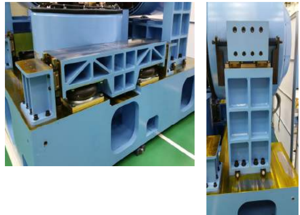
Fig.3 Floating Structure In Horizontal & Vertical
